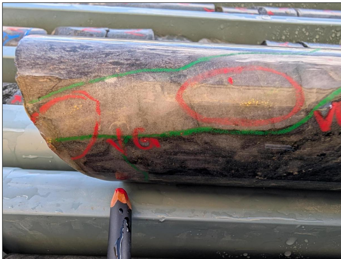
Figure 3 – Gold mineralisation located within a quartz vein hole 26HBBD044. The interval grades 4.20m @ 42.43g/t Au from 289.63m including 1.37m @ 126.93 g/t Au from 290.84m. Core width is NQ2 and ≈ 50.5mm in diameter for scale
