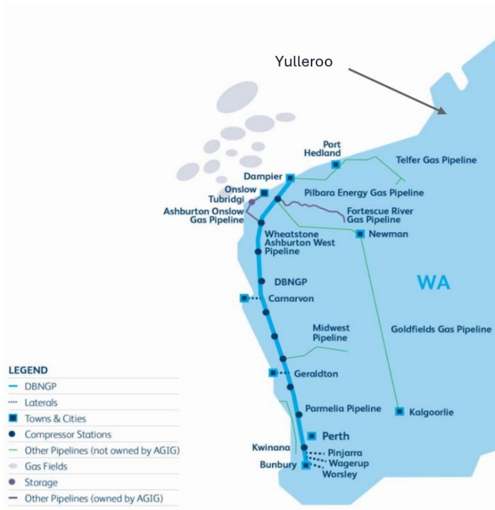
Figure 8 - Western Australia main pipeline infrastructure
