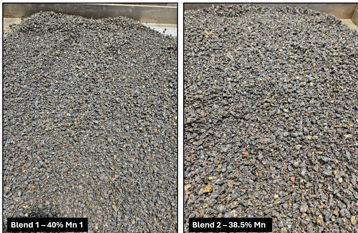
Figure 1. Blend 1 sinks at 2.8\text{g/cm}^3 - grade of 40.0% and Blend 2 - grade 38.5% Mn. Photo widths are about 40cm.
