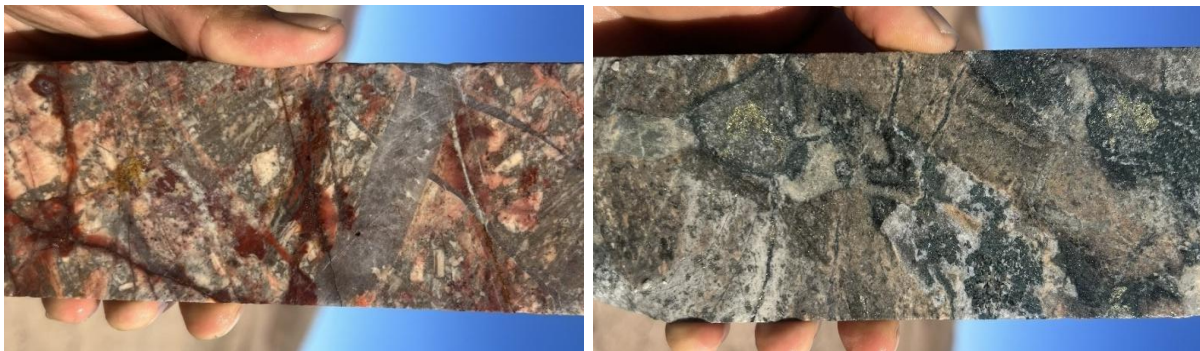
Figure 4: Core photos from CANDD003 showing breccias within the oxide zone with disseminated chalcocite (black) at 134m (LHS) – Breccia within the sulphide zone showing potassic alteration, chlorite muscovite veins with disseminated chalcopyrite at 382m (RHS).
