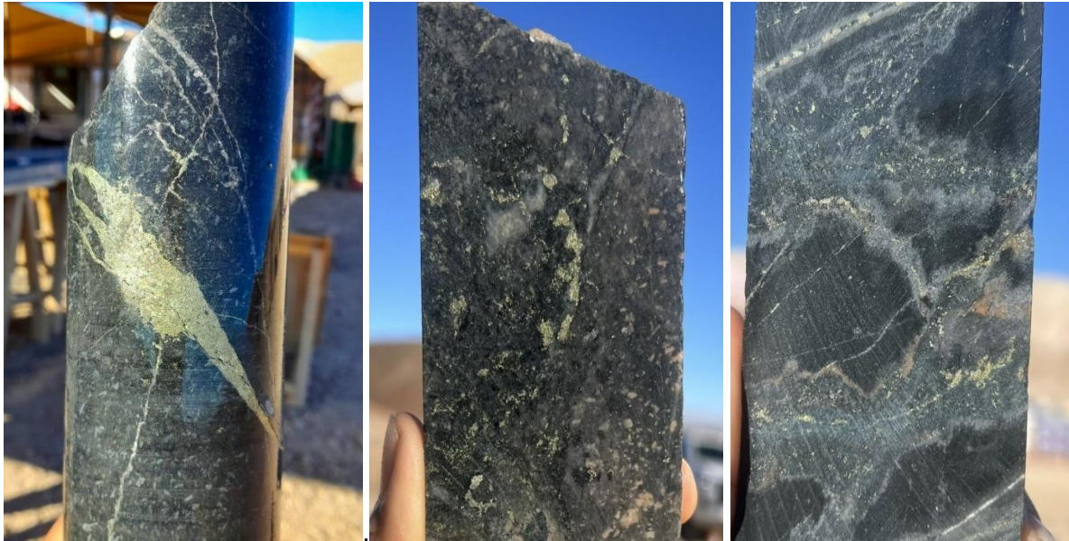
Figure 3: Core photos from CANDD003 showing chalcopyrite-filled veins at 308m (LHS) – disseminated chalcopyrite in porphyritic andesite host rock at 383m (centre); Muscovite-chlorite veins with K feldspar selvages and chalcopyrite either disseminated or forming centrelines in the veins at 504m (RHS).
