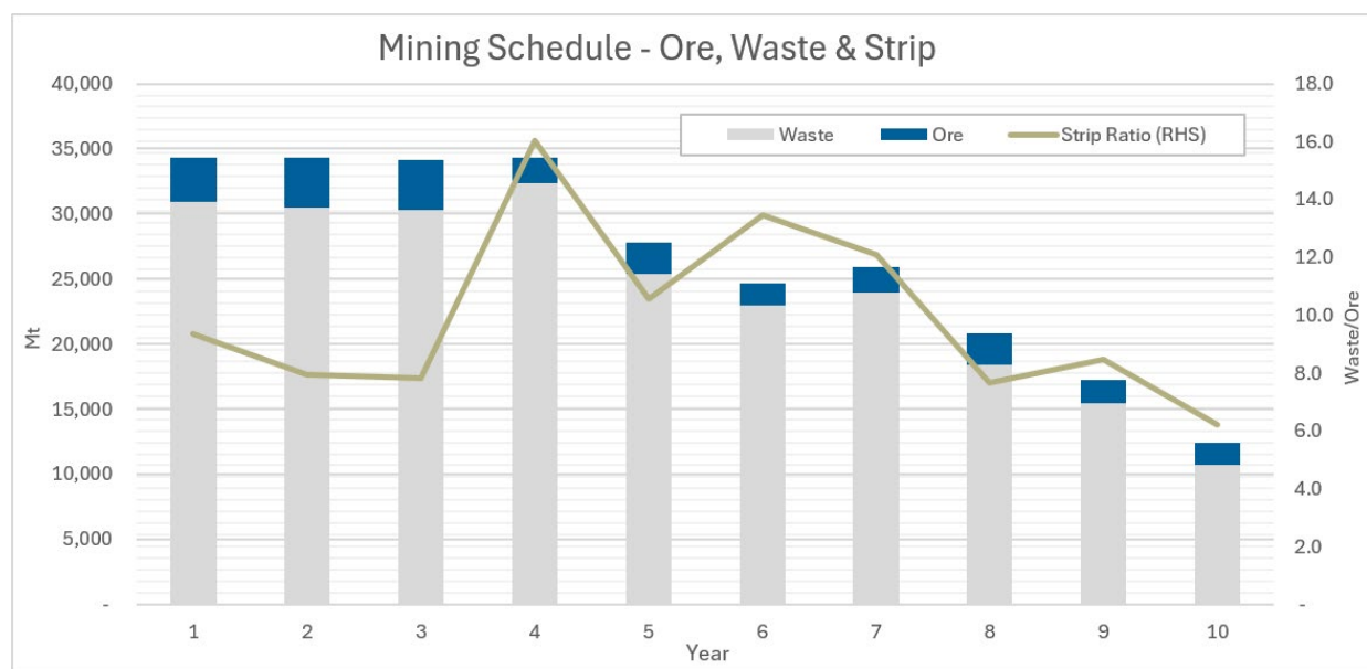
Figure 16: Mine schedule by material classification and strip ratio
