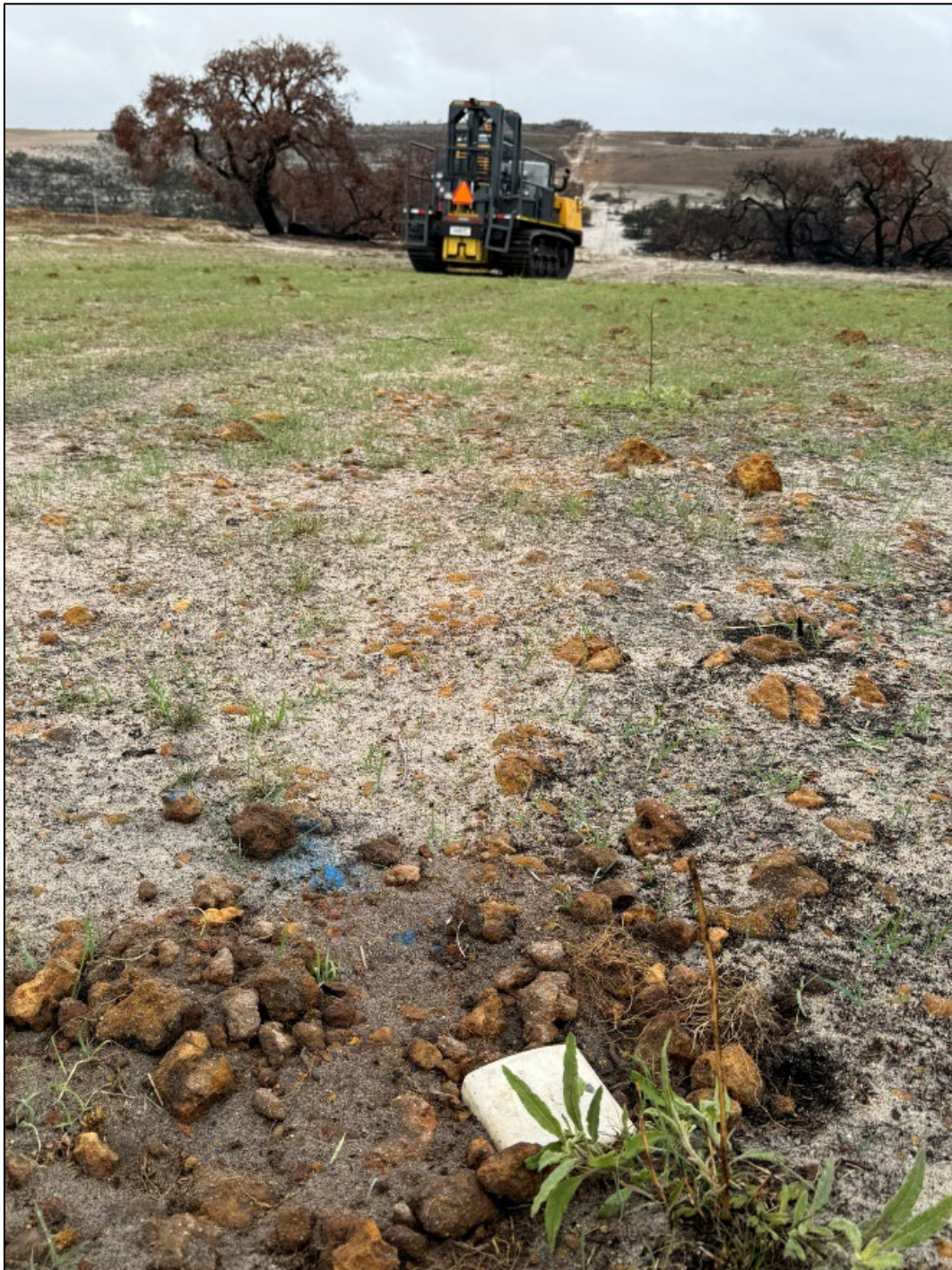
Figure 2. GeoPulse source vehicle and geophone recording the Barberton 3D seismic survey
