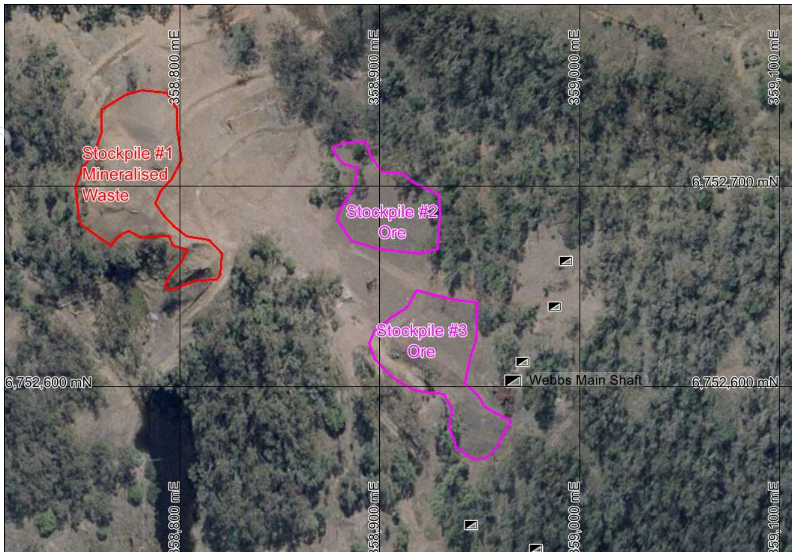
Sample Areas: WSHMM taken from red area – Stockpile #1 Mineralised waste; WPWHS taken from Ore Stockpiles #2 and #3
