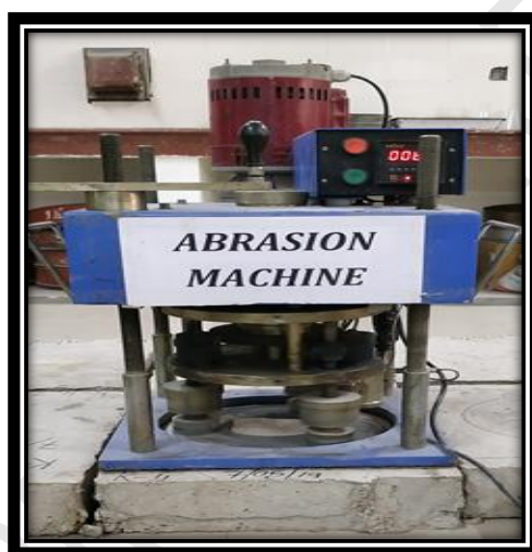
Fig. 9: Horizontal Concrete Slab under Abrasion Resistance Test
