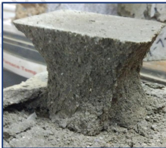
Fig. 1: A typical view of the Cement Mortar Cube after Test
