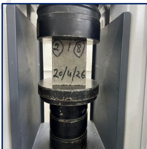
Fig. 3: A typical view of Compressive Strength Test in progress
