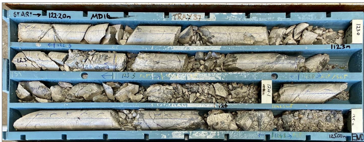
Figure 7.4 Example of LSR drill core showing extensive stockwork-like veins from hole MD16 (Tray #37), 122.2 m to 125 m; poor core quality is noted
