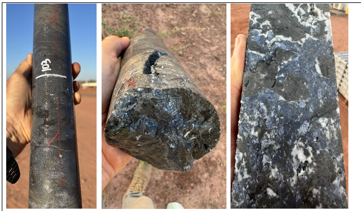
Figure 5: Photographs of drill core SHSD_214 (RHS) and SHSD_216 (LHS and centre) illustrating the style of galena mineralisation intersected at Omega North and at Norton. Note: Table 1 provides detailed ore-sulphides estimates for the references drill intervals.
