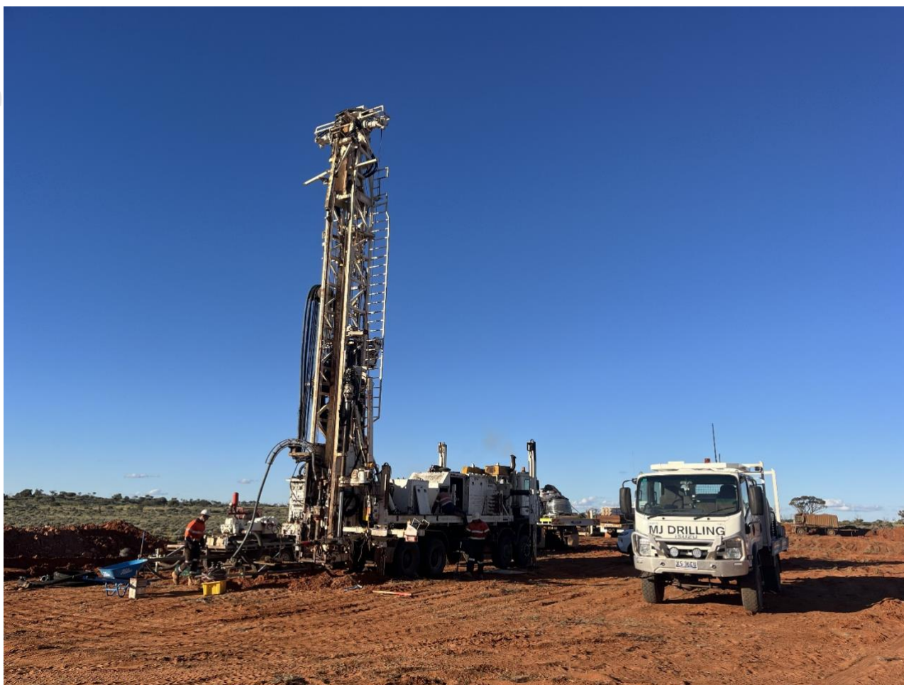
Figure 2 Drill rig mobilised for the hydrogeological programme at Elizabeth Creek.
