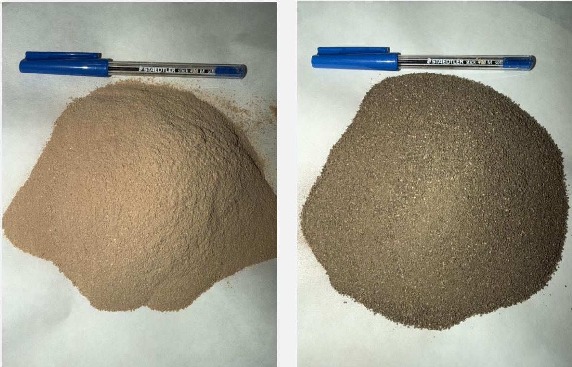
Figure 2. Heavy rare earth cleaner sample (right) produced at the North Stanmore pilot plant and (left) first rougher feed sample (Staedtler pen shown for scale).
