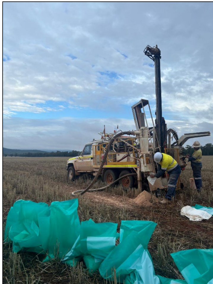
Figure 12: Aircore drilling at Tooronga during the quarter
