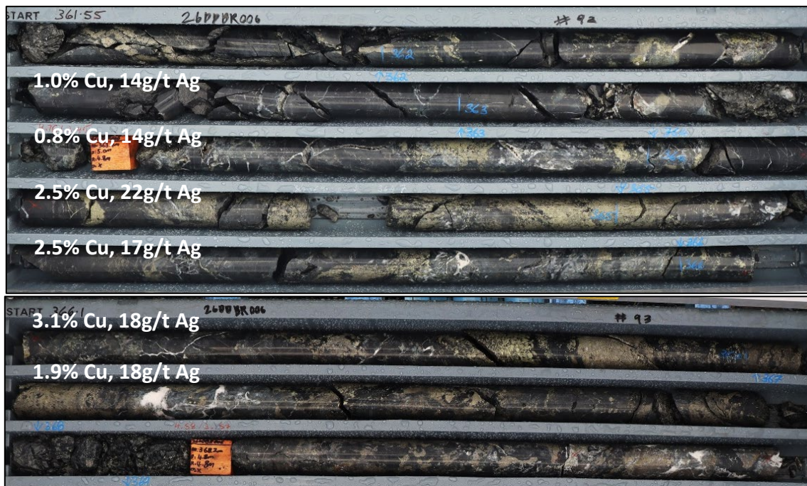
Figure 10: Semi-massive chalcopyrite mineralisation within the 35m mineralised zone intersected in 26DDBR006. The zone in this photo returned 6m at 2.0% Cu & 17g/t Ag from 362m
