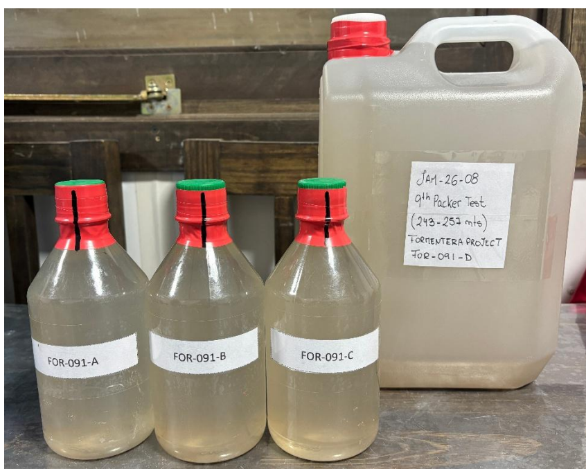
Figure 4. Brine Samples taken for lithium assay from packer test 9.
