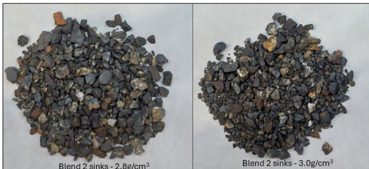
Figure 4. Blend 2 sinks at 2.8g/cm 3 and 3.0g/cm 3 with grades of 41.1% and 43.8% Mn respectively. Pile width is about 15cm.
