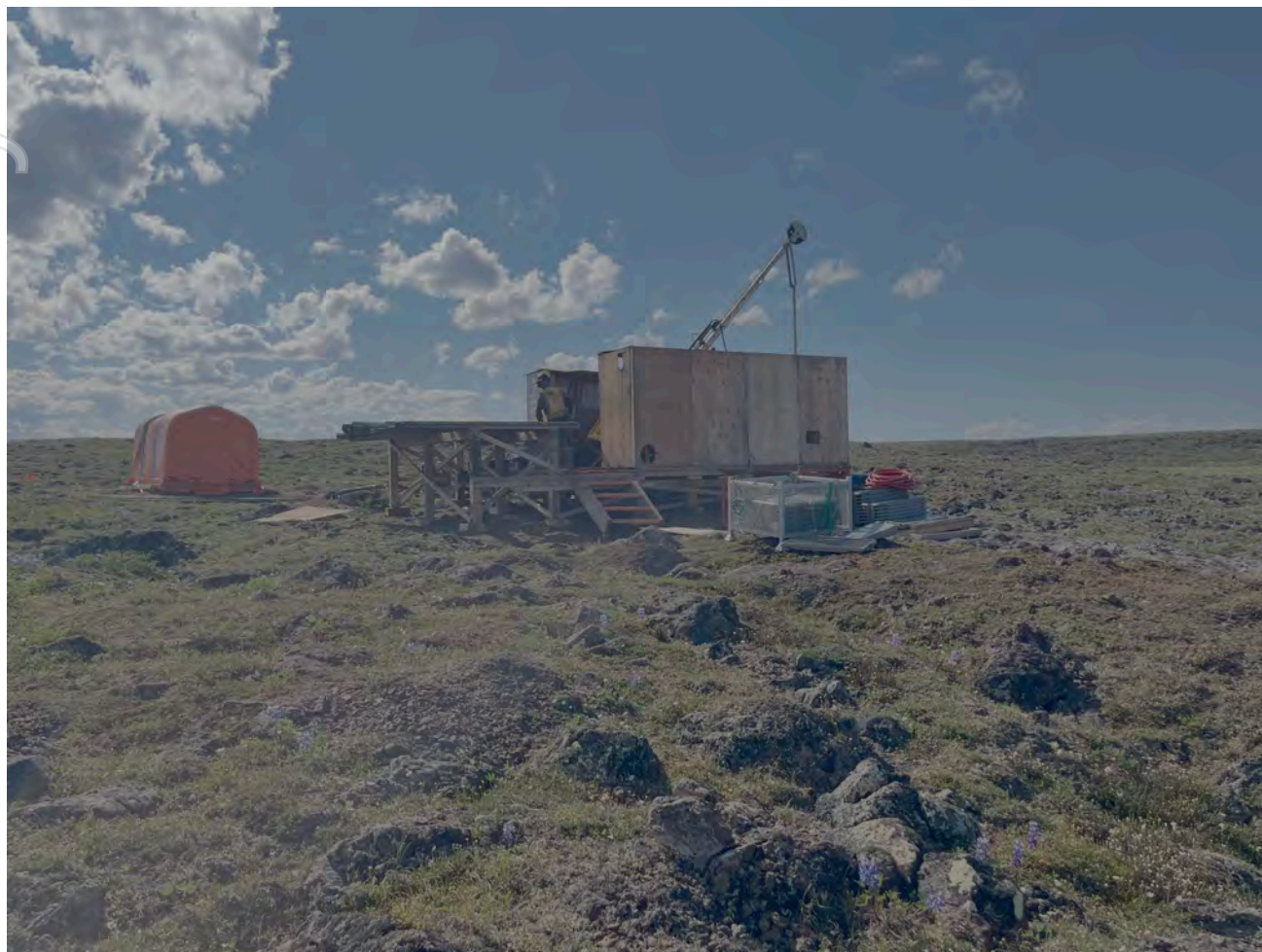
Figure 6 - Diamond Rig at Drill hole DAN26026.
