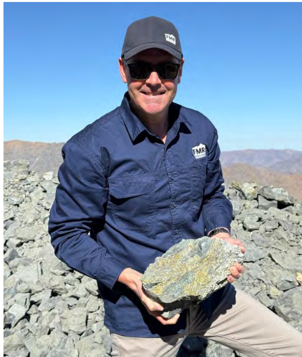
Photo 1. FMR Managing Director Oliver Kiddie, holding an underground sample from the La Martuca Prospect within the La Lorena Project, showing copper sulphide hosted in structurally controlled quartz-sulphide veining (see Appendix 2).
