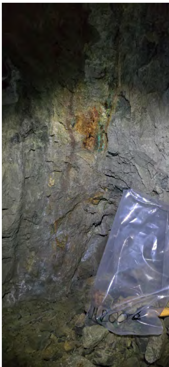
Photo 3. Underground rock chip sample 26MLR00006 from the La Martuca Prospect, showing copper oxide after sulphide associated with structurally controlled quartz-sulphide veining (see Appendix 2).
