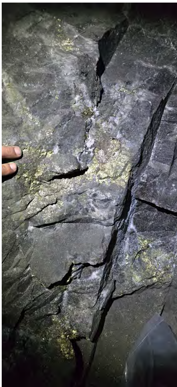
Photo 4. Underground mineralisation from the Los Morados Prospect, showing copper sulphide hosted in structurally controlled quartz-sulphide veining (see Appendix 2).
