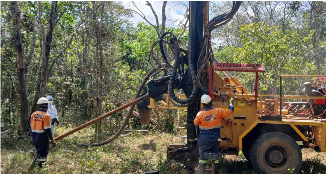
Figure 4: AC drilling at West Mwombezhi
