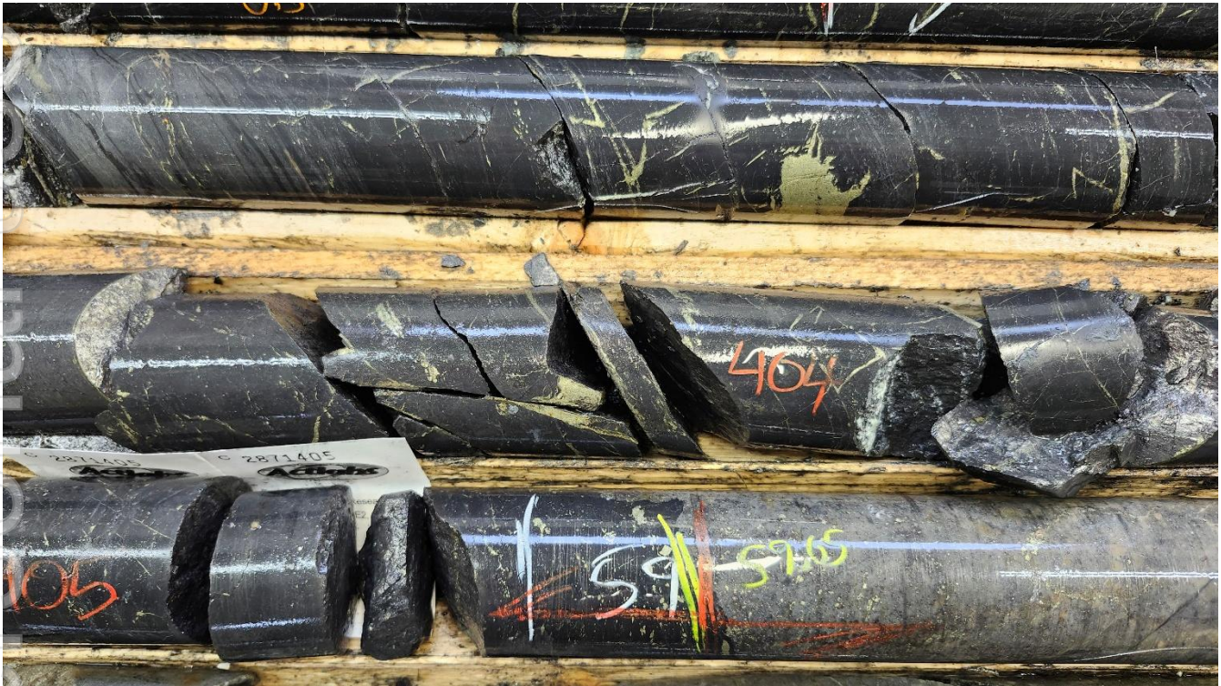
Photograph 2: TX26-005 Diamond Drilling Core, Mineralised Porphyry/Argillite Contact @59m Depth
