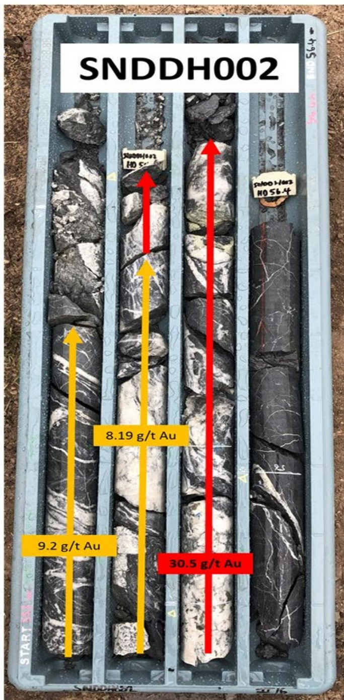
Figure 2: High-grade core from diamond drill hole SNDDH002. (ASX: FAU, 10 June 2021) 4
