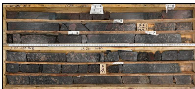
Figure 2: Drill core from hole L26-688 showing part of the mineralised zone (25.1m to 31.6m) reporting 2.1% TREO. The dark, largely chlorite alteration is characteristic, while remnant, pink coloured feldspar grains are noted.
