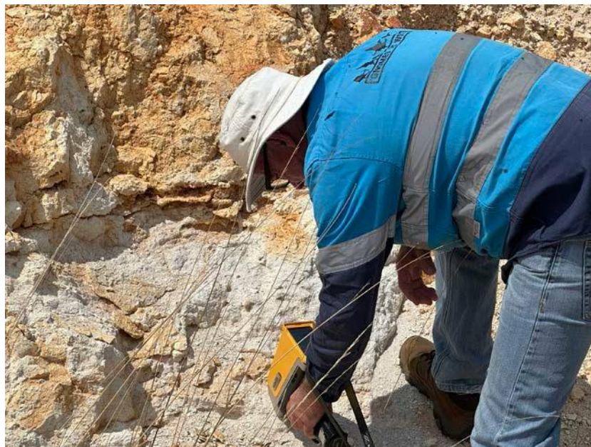
Figure 9 REE Target - pXRF sampling of white weathered kaolinitic fine-grained sediments adjacent to the prominent scarp as shown in Figure 12
