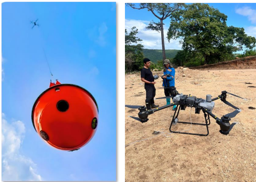
Figure 4. UAV sling mounted MobileMTd Sensor and FlyCart30 heavy-lift Quadcopter
