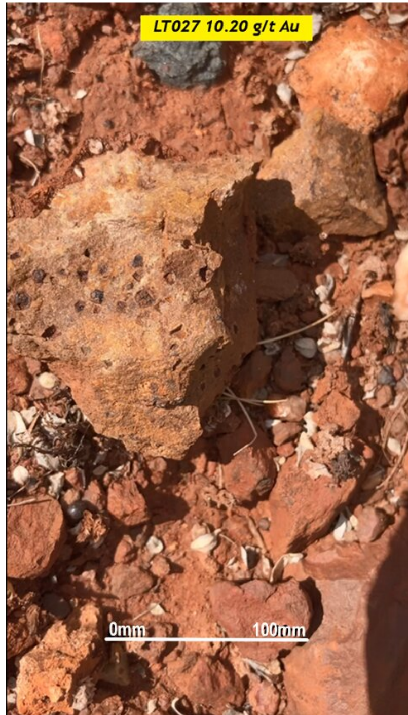
Figure 2 Rock sample LT027 displaying Euohedral sulphide casts providing a gold grade of 10.20 g/t Au
