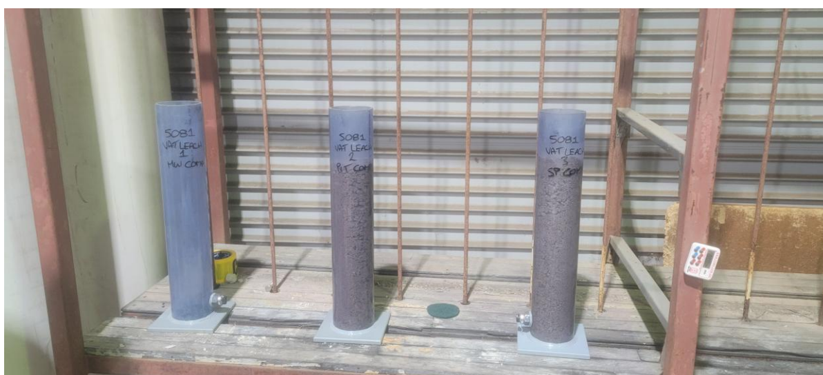
Figure 3 Agglomeration & percolation and Column Leach Test work at Bureau Veritas lab Perth.
