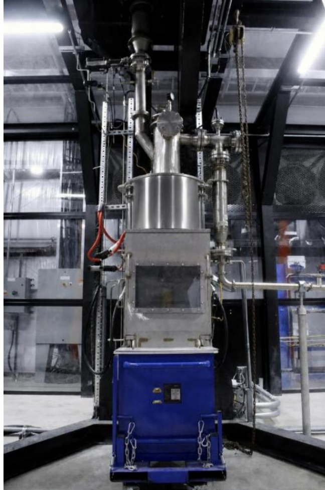
Figure 8: Latest iteration of Metallium's commercial scale semi-batch reactor representing a 400,000x scale-up
