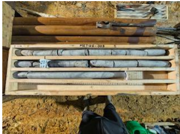
Fig 4: Excellent core recovery from initial drilling
