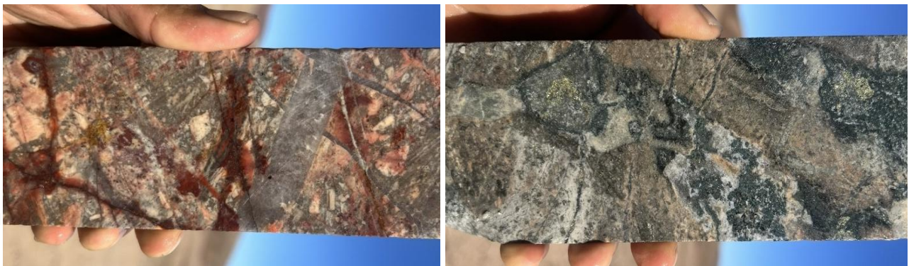
Figure 6: Core photos from CANDD003 showing breccias within the oxide zone with disseminated chalcocite (black) at 134m (LHS) – Breccia within the sulphide zone showing potassic alteration, chlorite muscovite veins with disseminated chalcopyrite at 382m (RHS).
