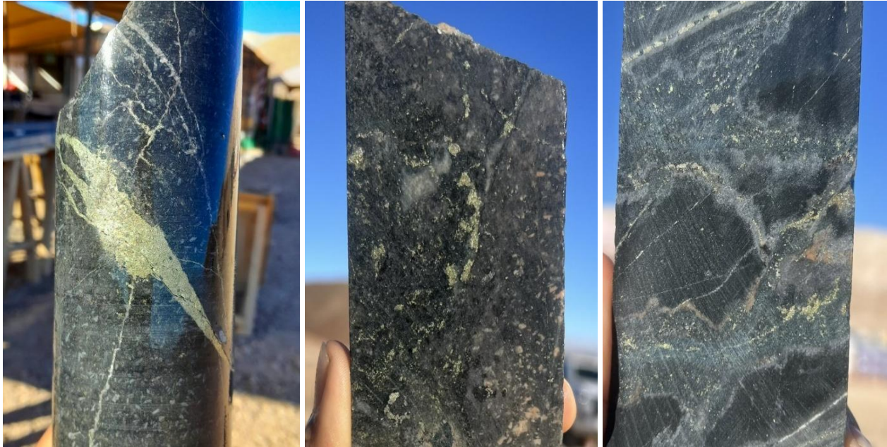
Figure 5: Core photos from CANDD003 showing chalcopyrite-filled veins at 308m (LHS) – disseminated chalcopyrite in porphyritic andesite host rock at 383m (centre); Muscovite-chlorite veins with K feldspar selvages and chalcopyrite either disseminated or forming centrelines in the veins at 504m (RHS).
