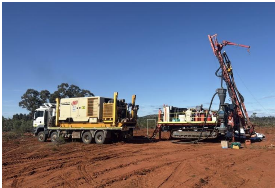
Figure 5. Dual purpose, track mounted rig that will shortly be mobilised to the Horn Island gold project
