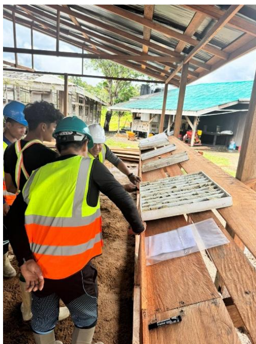
Figure 14: Core logging stands at NP with core shed team training geotechnical logging (left). Diamond drilling equipment and consumables ready for mobilization (right)
