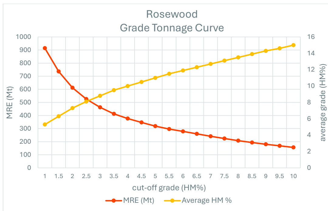
Figure 5: Rosewood Resource grade tonnage curve
