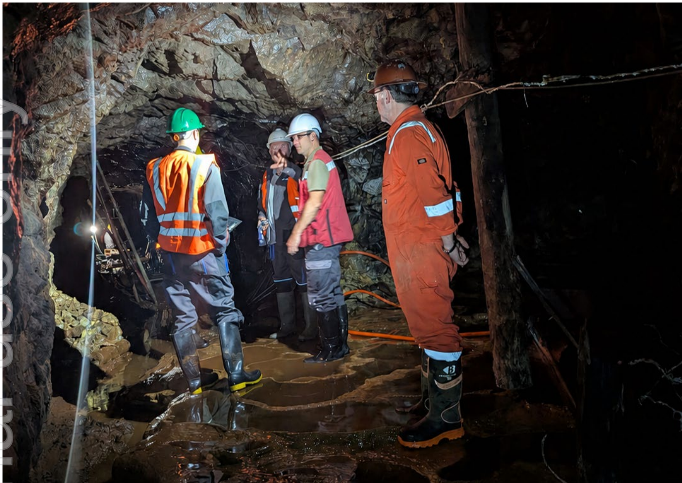
Figure 6 Resource and mining consultants inspecting the underground adits and vein exposure
