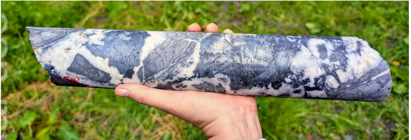
Figure 3 Photograph of 44cm long drill core from hole DD26ZOP-002 (interval 44.66 – 45.00m) showing stibnite (antimony mineral) (estimated ~25%), slate and quartz breccia with disseminated sulphides. Assays are pending for this interval. Visual estimates of mineral abundance should never be considered a proxy or substitute for laboratory analyses where concentrations or grades are the factor of principal economic interest. Visual estimates also potentially provide no information regarding impurities or deleterious physical properties relevant to valuations.
