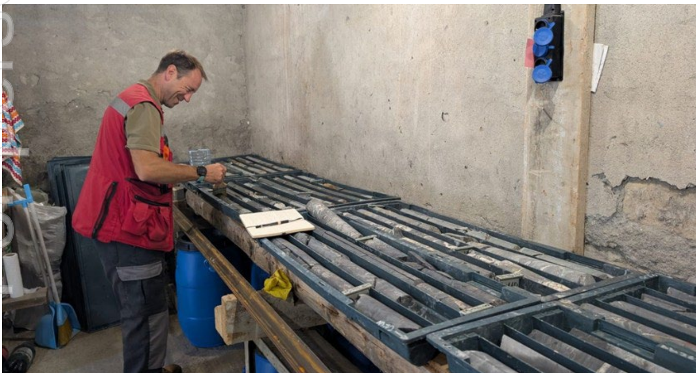
Figure 7 Photo of resource consultant geologist inspecting the core from 2025 and 2026 drill programs
