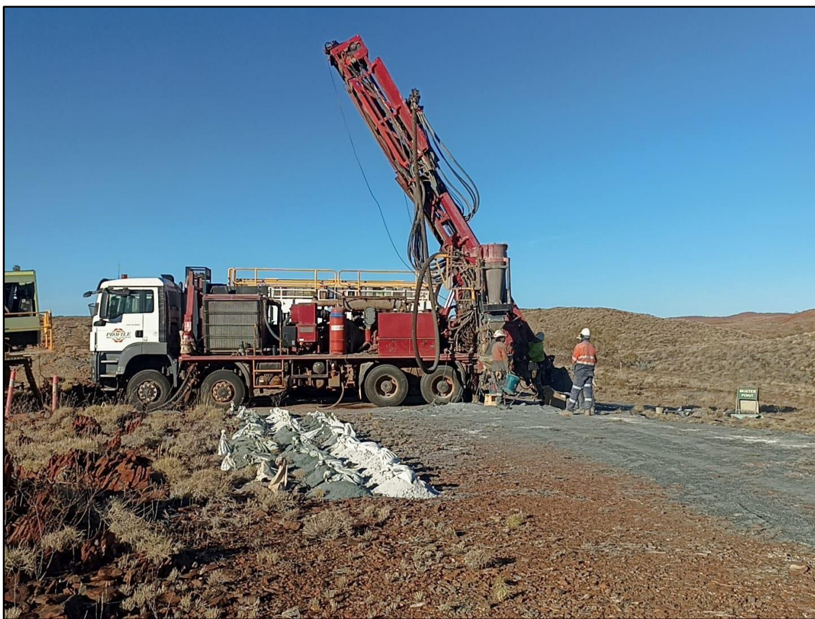
Figure 1 RC rig on-site at Tambourah King.
