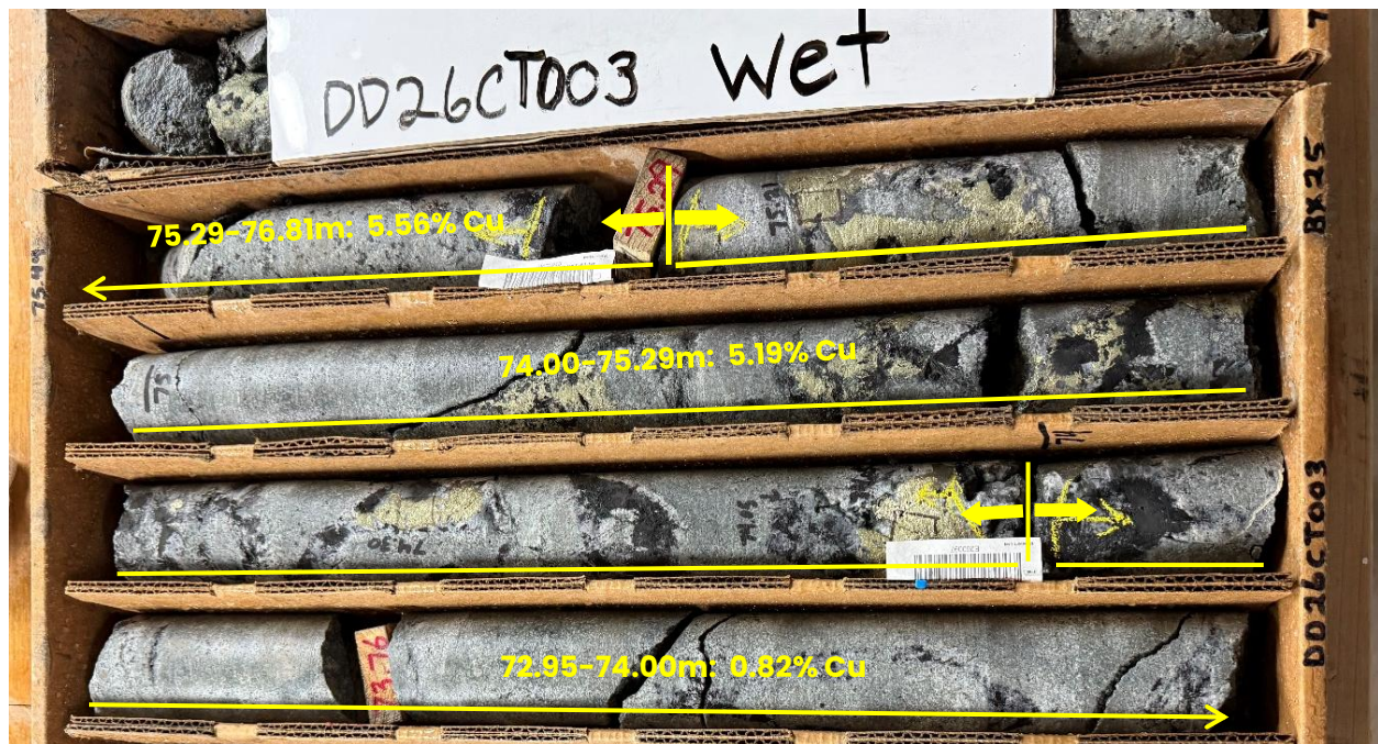
Figure 5: Chalcopyrite copper mineralisation in drill core from hole DD26CT003, Cactus Corridor.
