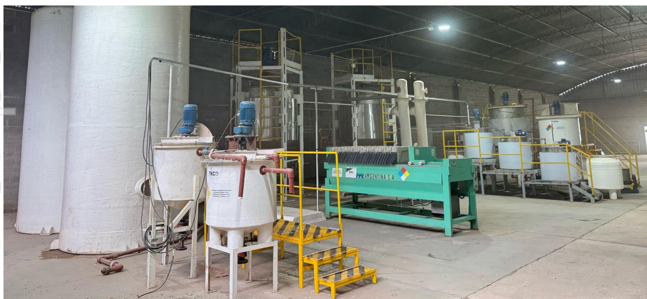
Figure 8: Pursuit's 250tpa Pilot Plant producing Lithium Carbonate in Salta, Argentina
