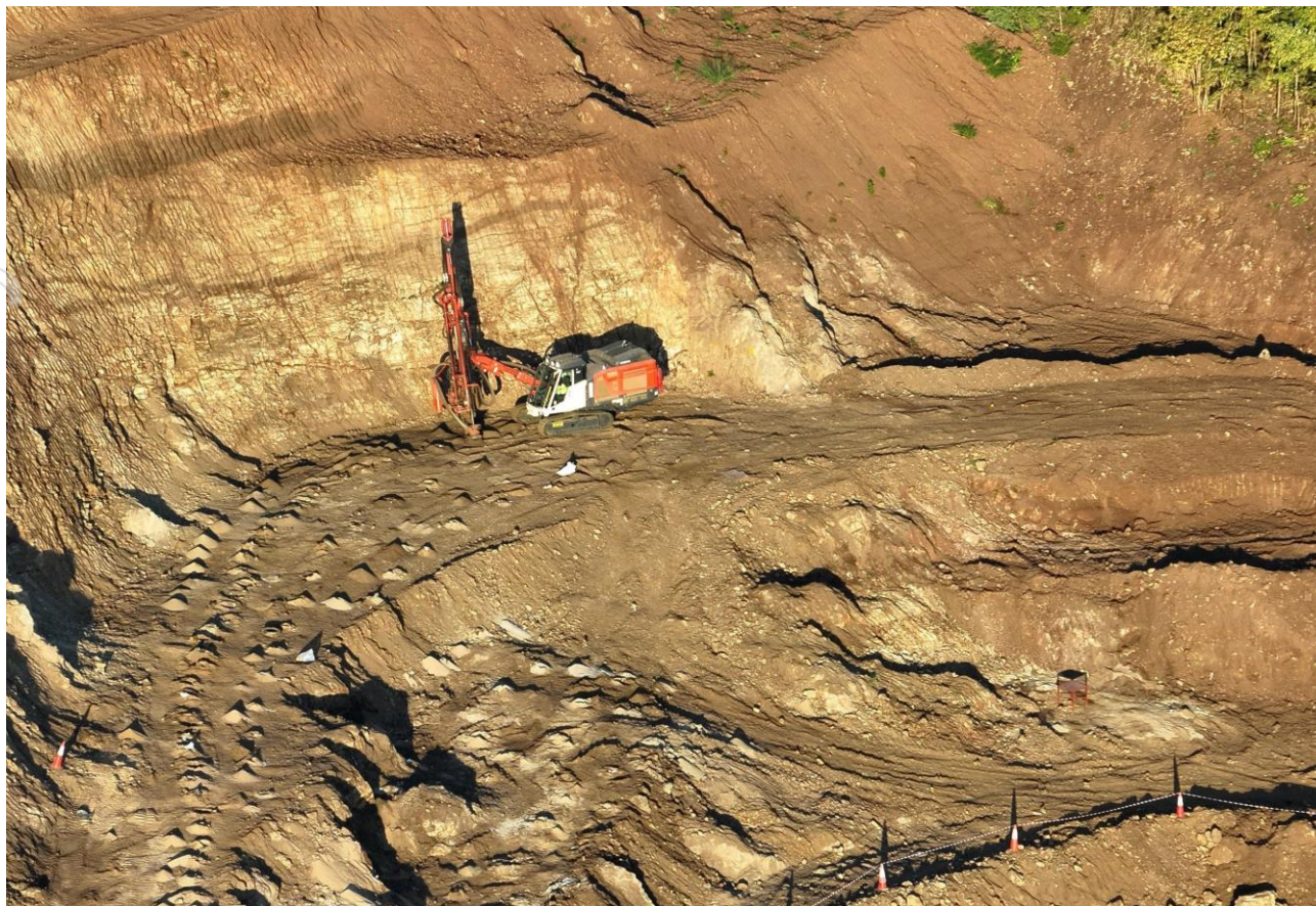
Picture 3. Production drill rig drilling the first blast pattern at the Stage 1 pit area, marking a key mining readiness milestone ahead of the planned first blast at Kangankunde
