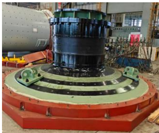
Figure 2: Ball mill shell (left) and head (right)
