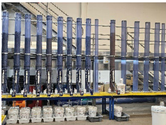
Plate 1: Apollo Hill Column Leach Variability Tests in Progress. Tests used to optimise Heap Leach process for the Apollo Hill Definitive Feasibility Study.
