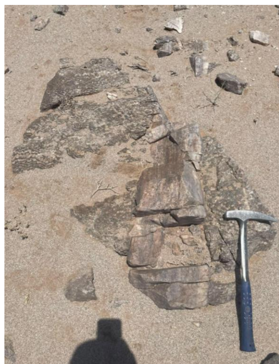
Figure 7 High-level carapace architecture at Sukhaybarat South. Highly fractionated magma indicators (unidirectional solidification texture banding running left-to-right) are overprinted and crosscut by banded quartz veins - a magmatic relationship indicative of a volatile-rich, prospective IRG style mineralised system.
