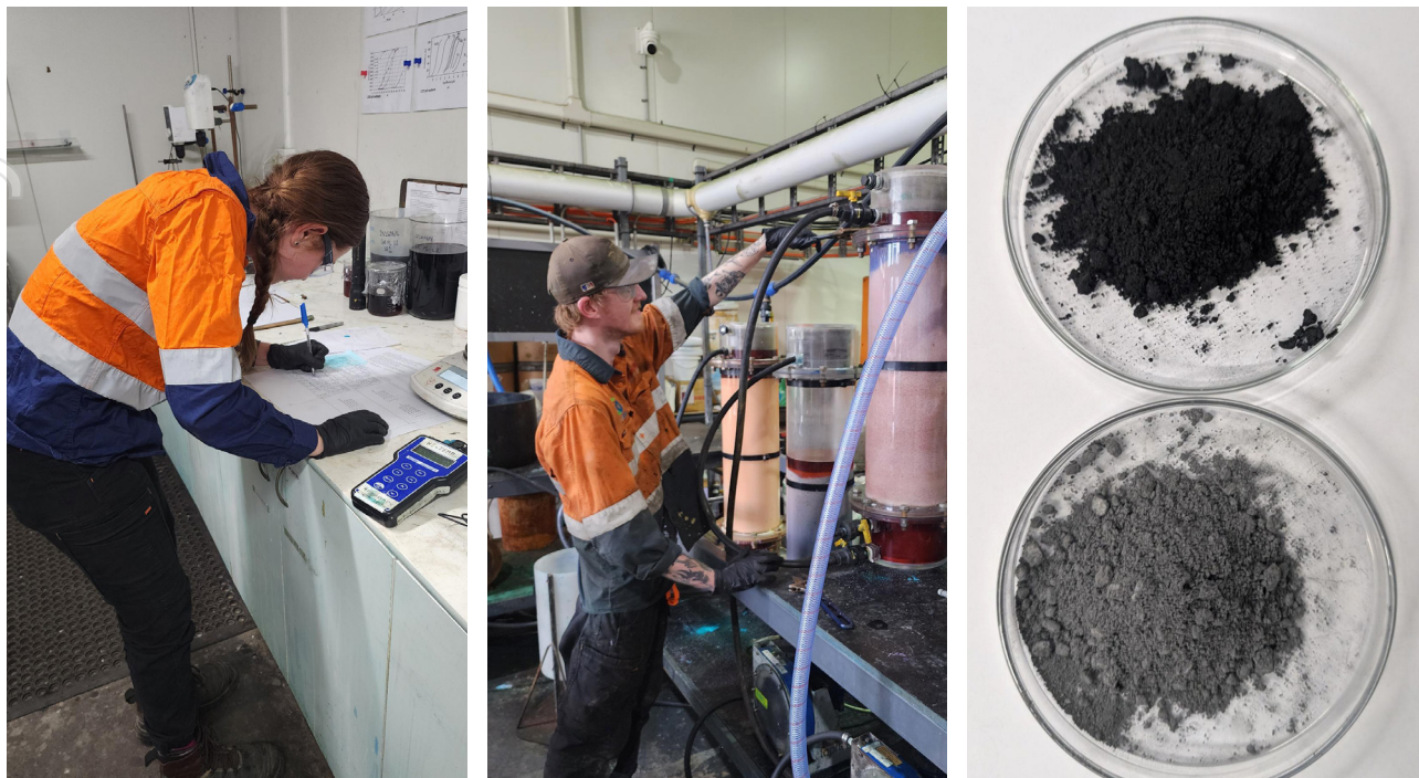
Figure 2 – Left and centre: Testwork activities undertaken by staff at the BHCP Technology Centre (BHTC). Right: Graphite-rich concentrate recovered by flotation from battery black-mass leach residue (top), and the remaining gypsum-bearing flotation tailings (bottom). Source: Cobalt Blue Holdings Limited.
