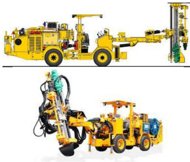
Image 4: Muki Production Drilling Rig, to be used at the Reward Gold Mine
