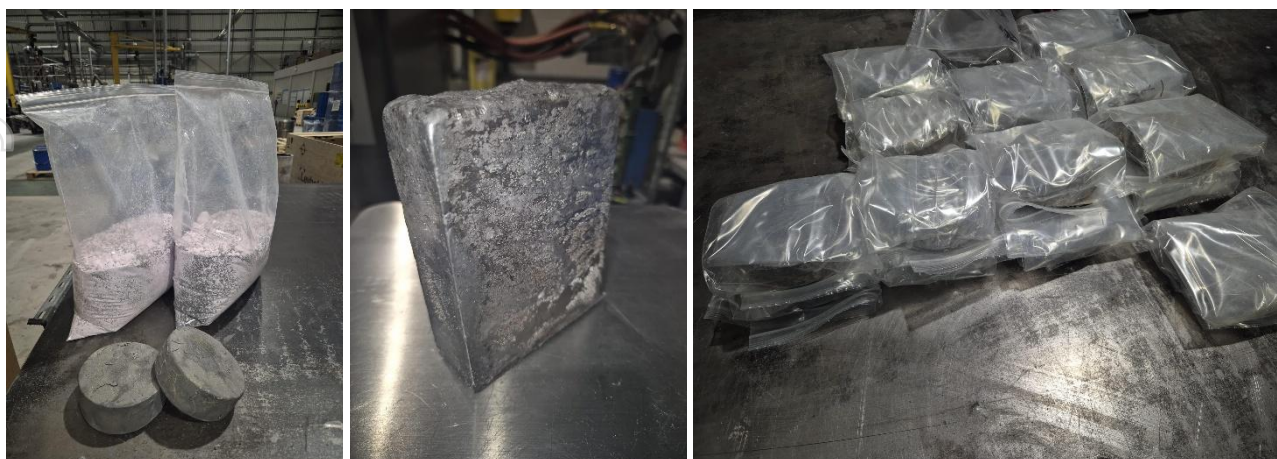
Figure 1: Neodymium ingots after reduction; Dysprosium (centre) and Terbium ingots (right) after Vacuum remelting (used with permission from LCM).
