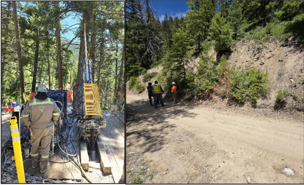
Figure 7: LEFT: Drilling Rig 03 (Left) at hole HH-GG26-004 on Ds10; RIGHT: Ds8 after drilling is completed. Three holes were drilled on Ds8 (HH-GG26-010, (HH-GG26-011, and (HH-GG26-012). Taking advance of the placing the drill sites on and very close to the access tracks, the rehabilitation is such that there is no visible trace of the drill collars.
