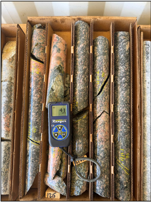
Figure 3: CE26-05 - 1215-1217 feet – interstitial calcite
