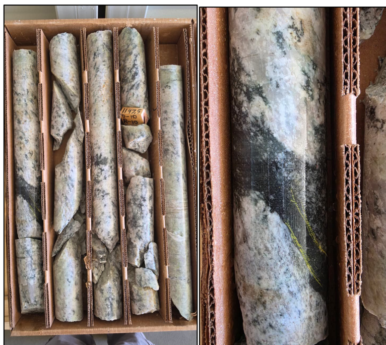
Figure 5: CE26-16: 1141.5 feet - biotite rich section within hydrothermal intrusion with moderate radioactivity.
