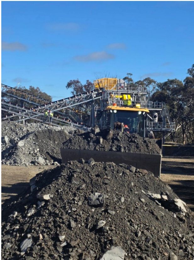
Figure 2 Ore loading on ROM (run of mine) pad
