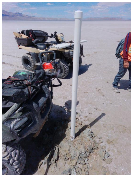
Figure 16: Hand Auger drill hole recently completed at White Plains Lithium Brine Project
