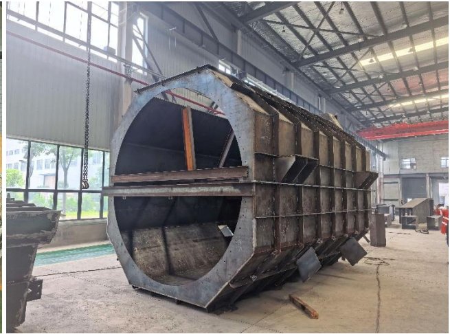
Photos 11 & 12: Completed plant hopper (LHS) and mill trommel cover (RHS)
