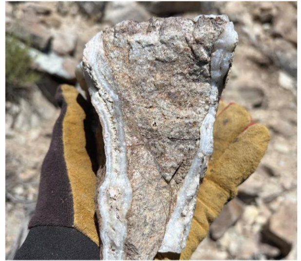
Figure 5: Hand specimen from TUC showing low pressure, low temperature quartz veins in a breccia zone around altered granite clasts.
