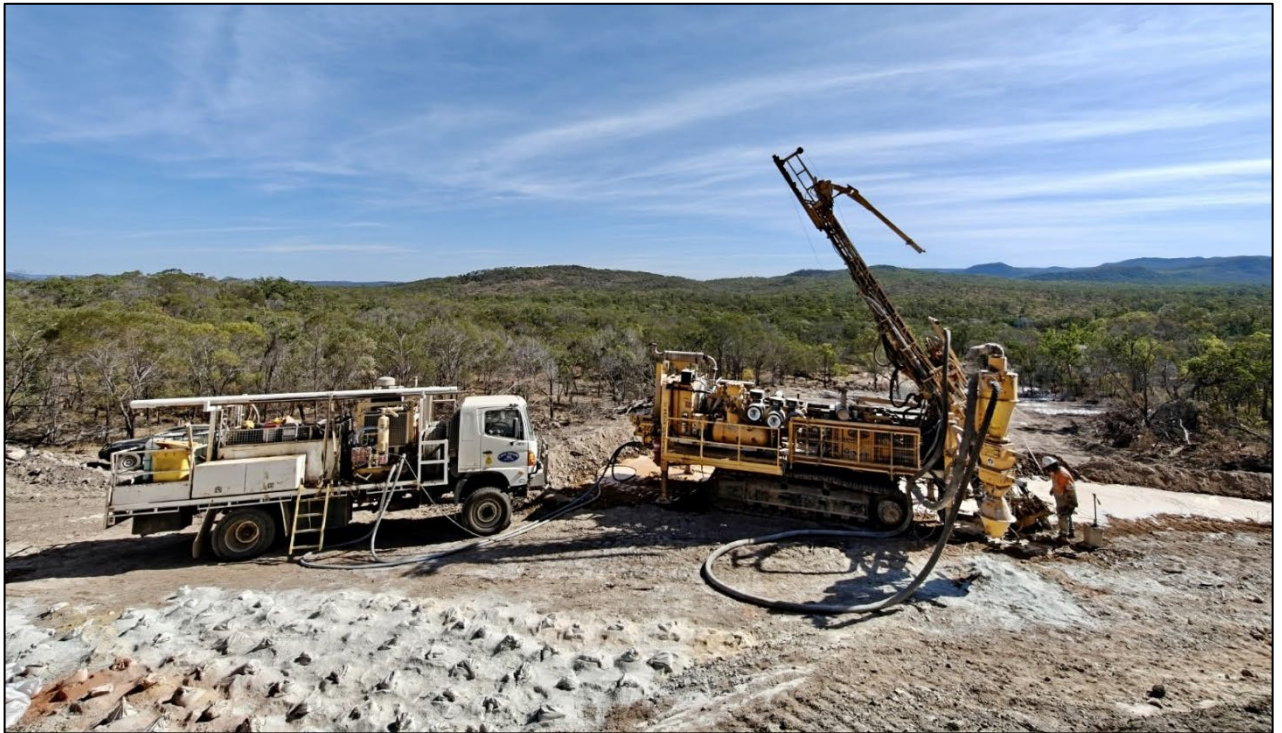
Figure 1: RC rig drilling Francis Creek East, Sybil.
