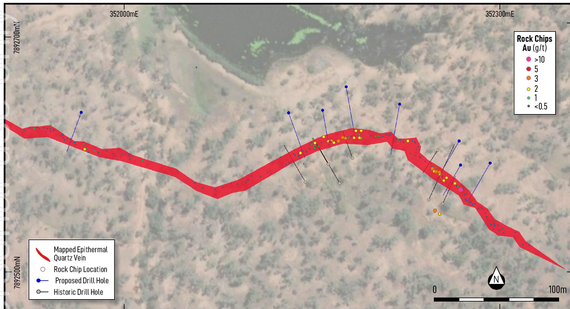
Figure 7: Planned drill program at Blue Range comprises 8 holes (~375m drilling).
