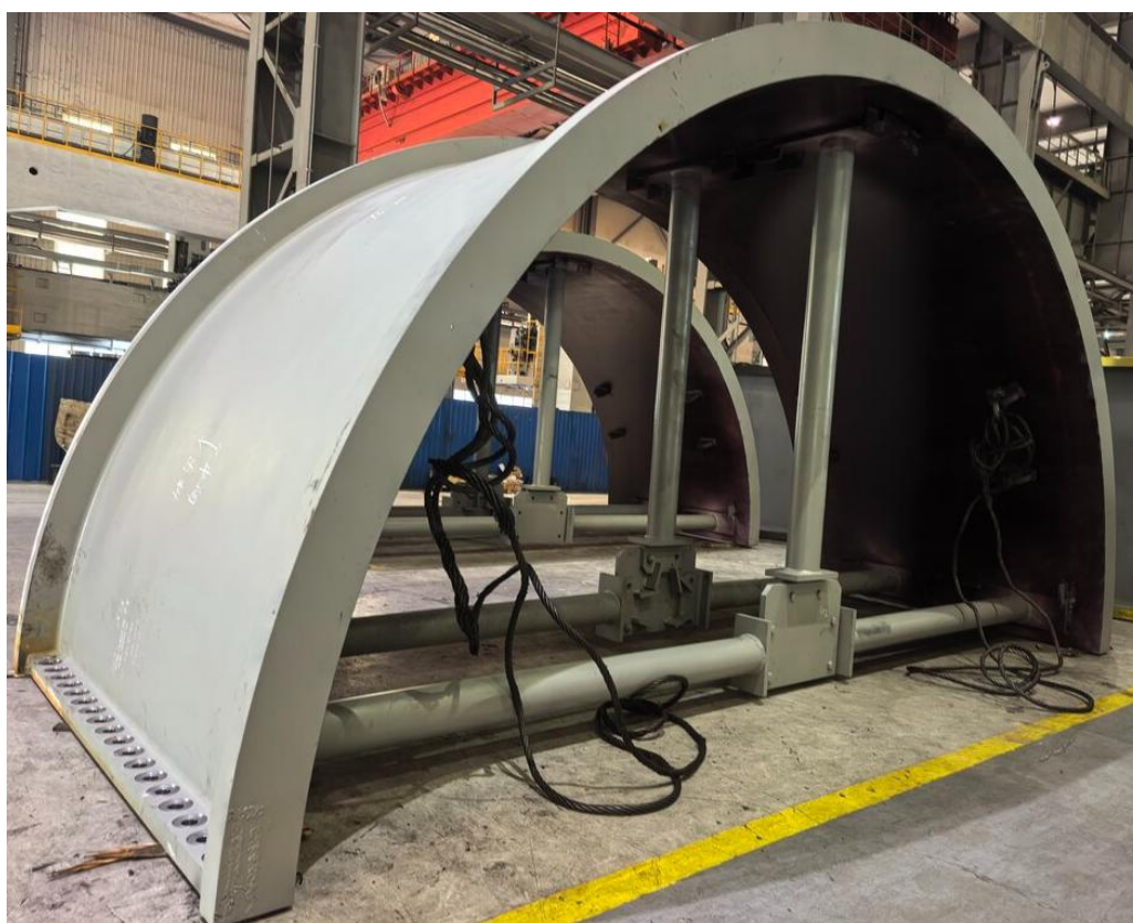
Figure 6 – SAG mill shells being fabricated
